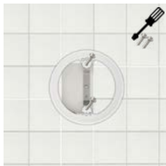
3. Place the ring on the recessed housing and screw it to recessed housing.
