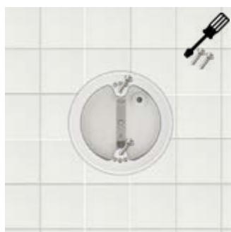
7. Fill the edge with cement/tile adhesive and screw the ring back onto the recessed housing so that it is flush with the surface of the tiles. The ring can then be added flush with the other tiles.
