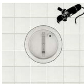
6. Remove the tiles, grind the tiles to the desired shape and stick them back.
