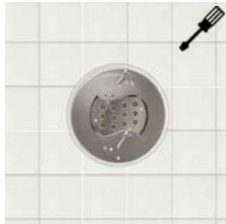
4. Place the pool light and tighten the screws.
